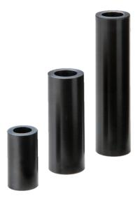
EKK manufactures carbon materials for bush / bearings. The in-house material capabilities include the blending of carbon graphite with resin, hot molding, sintering, and heat treatment at high temperature.
